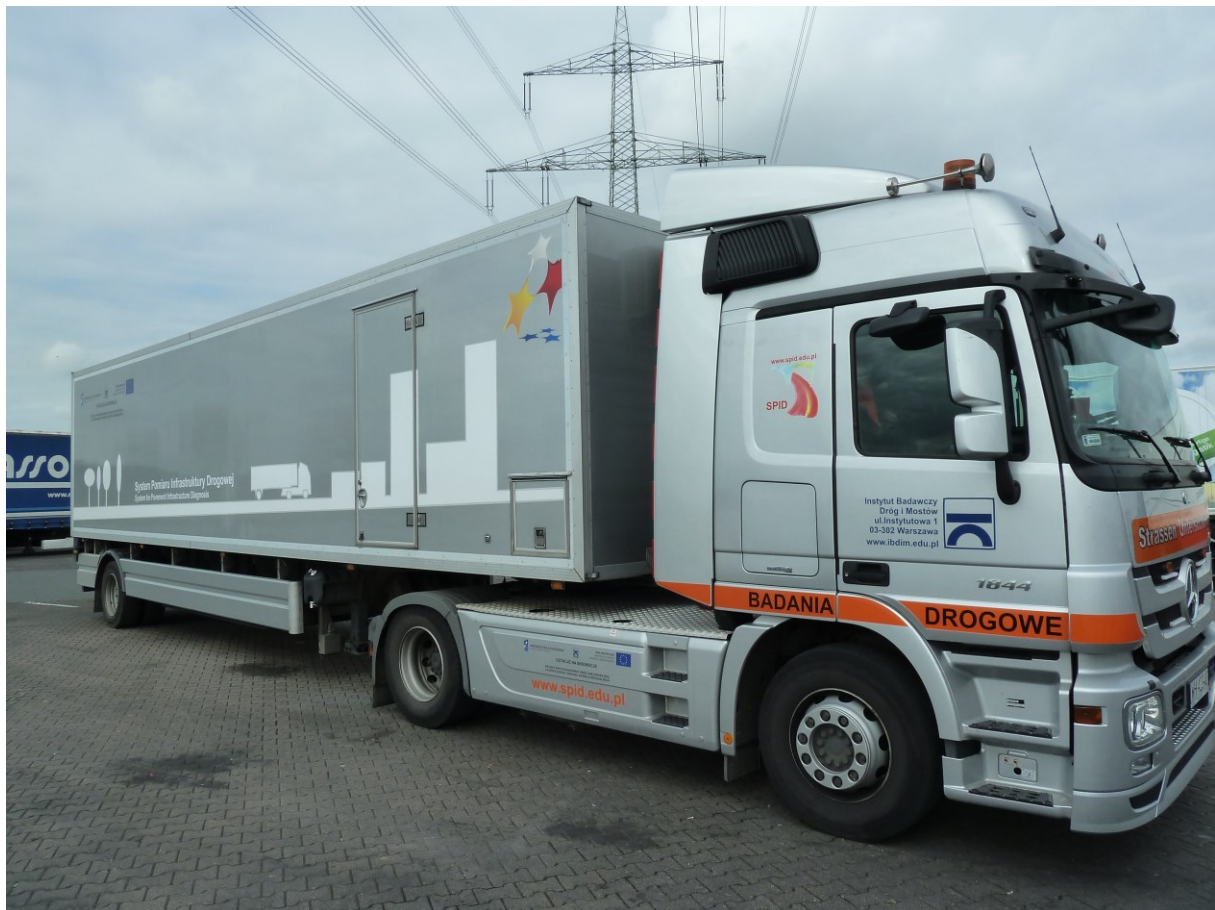
Abbildung 5: Traffic Speed Deflectometer (TSD) des Road and Bridge Research Institute in Warschau
